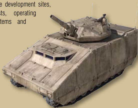
Figure 1 The Non-Line-Of-Site Mortar (NLOS-M) vehicle, as depicted in this artist's rendering, is one of the 18 combat systems that comprise the Army's Future Combat Systems. (U.S. Army image.)
